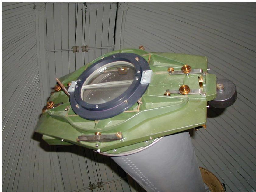
Fig. 4.8 – Objetiva do heliômetro do Observatório Kuffner (Áustria). Foto: Martin Sloboda - Kuffner-Sternwarte. [http://kuffner-sternwarte.at/sternwarte/vks\\_ksw\\_instr1.php](http://kuffner-sternwarte.at/sternwarte/vks_ksw_instr1.php)
